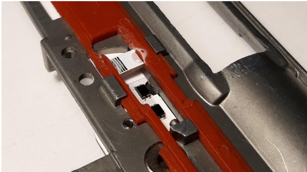
Selector plate insert is to the left of the semi sensor.
